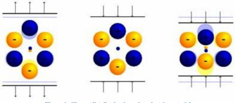
Figure 1: Charge distribution in a piezoelectric material
